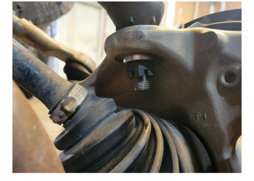
**Step 5. (Install Upper Control Arm Into the Hub Assembly)** Remove the cotter pin and castle nut from the Moog upper ball joint and install it into the hub assembly. Make sure to only tighten the castle nut hand tight until front installation is complete and desired camber is achieved. Do not install cotter pin at this time.
