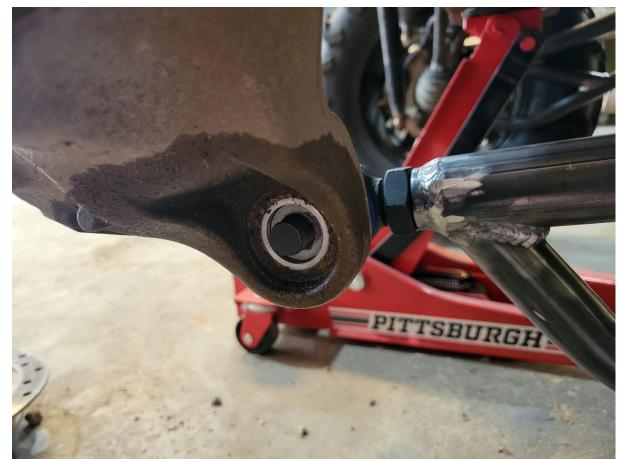
Using the stock hardware, reinstall your new TTC Arms back on the machine and repeat on other side.
