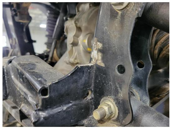
**Step 3. (Finish Installation)** Once the receiver gusset is trimmed and the bumper fits without interference, dust a few sprays of black paint on the bare metal area of the frame that was just trimmed, and finish installing the bumper with the existing hardware. You will reuse all of the factory bolts that hold the cage to the frame. Sometimes it is necessary to use an alignment pin to get the holes to line up to install the bolts.
