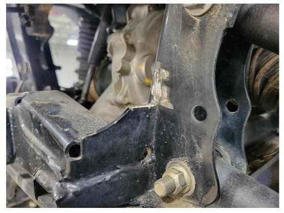
**Step 3. (Finish Installation)** Once the receiver gusset is trimmed and the bumper fits without interference, dust a few sprays of black paint on the bare metal area of the frame that was just trimmed, and finish installing the bumper with the supplied hardware.
