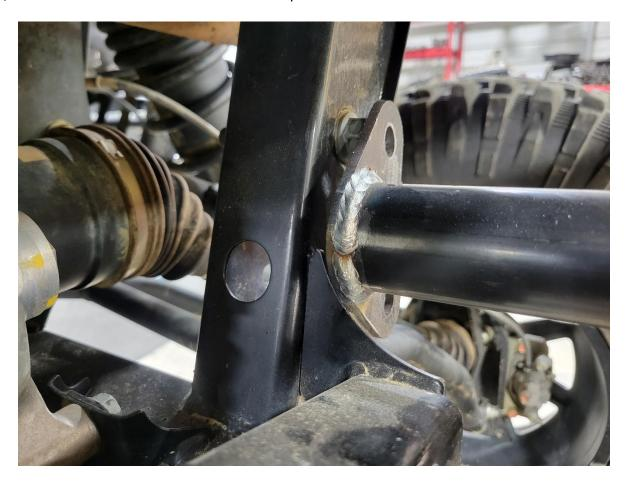
**Step 2. (Trim Receiver Hitch Gusset)** If your model has gussets that interfere with the bumper, you will need to trim the top part of the gusset off for clearance. Mark the gusset like the picture below and trim with a cutoff wheel, grinding disk, or Sawzall.
