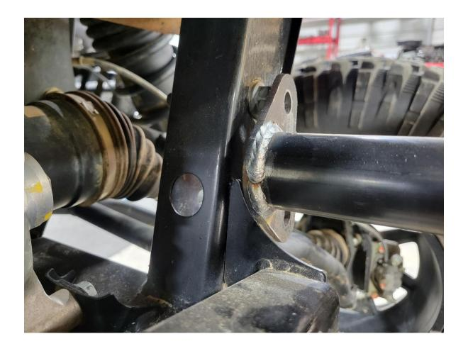
**Step 2. (Trim Receiver Hitch Gusset)** If your model has gussets that interfere with the bumper, you will need to trim the top part of the gusset off for clearance. Mark the gusset like the picture below and trim with a cutoff wheel, grinding disk, or Sawzall.
