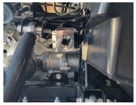
Next, make sure the jam nut is not installed on the inner tie rod (or heim joint), and push your stock tie rod boot on to the 14 mm shaft of the inner tie rod end, then screw on the jam nut.
