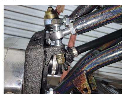
**Step 9. (Tighten Frame Bolts)** Once everything is assembled hand tight, go ahead and fully tighten both the upper and lower frame bolts that mount the control arms to the frame.
