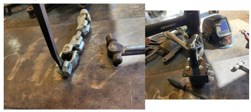
**Step 3.** Now assemble the Orbital valve in this order, **steering column, bracket spacer, frame bracket**. For now, leave the bolts hand tight. Install and tighten the 4 fittings into the Orbital valve at this time.
