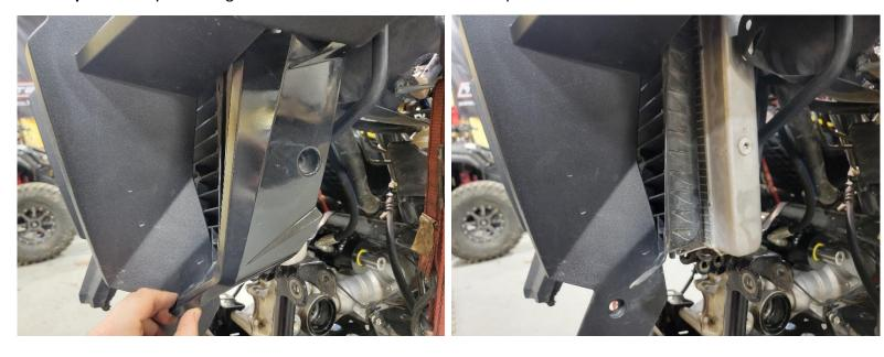
**Step 2.** Next push the lower grill pegs out of the radiator mounting holes on both sides as shown below.
