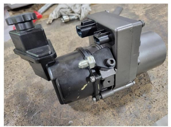
Step 2. Now install the TTC pump bracket to the frame as shown below, then bolt the pump to the Bracket.
