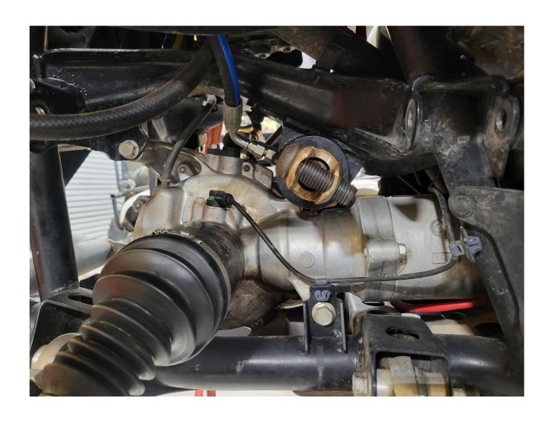
Ideally you want to line the clevis "ears" up with the hole in the hub assembly where the outer tie rod will attach. See pic below.
