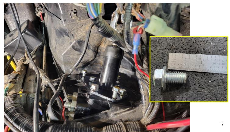
**Step 6.** Once everything is in place, tighten down the 3 bolts that secure the orbital valve bracket to the frame. Then tighten down the 4 bolts that hold the bracket and steering column to the orbital valve. **(Don't worry about whether your steering wheel is straight or not at this time)**
