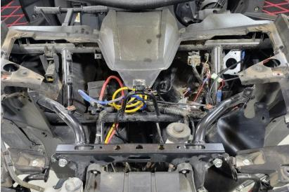
**Step 2.** Now that you have access to the EPS unit, remove the bolt that secures the steering yolk to EPS unit and the bolt that holds the yolk to the upper steering shaft. This will make it easier to remove the EPS Unit.
