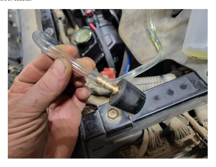
Apply 15-18 inches of vacuum to the system. With the pump on, turn the wheel lock to lock, holding at full lock for no more than 2 seconds before turning back the other way. Do this until no more bubbles are occurring.
