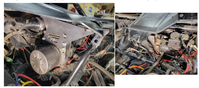
**Step 3.** Next, locate the pump to orbital valve hose shown below. First connect one end to the orbital valve and tighten down. Route the other end up to pump area. At this time go ahead and connect the hose barb from the Upper Fluid cooler hose to the last spot on the orbital valve and tighten down.
