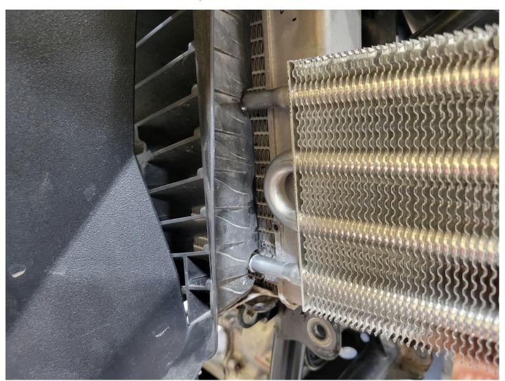
**Step 5.** Once the holes are trimmed, install the supplied hoses to the fluid cooler and put cooler into place for a test fit.
