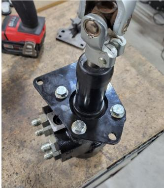
**Step 4.** Now install the Orbital valve assembly into the machine. Once you get the Orbital valve assembly in place, connect the yoke to the steering column before you start any of the frame bolts. Make sure to line up the yolk with the flat spot on the steering shaft so that the 10mm retaining bolt will install properly.
