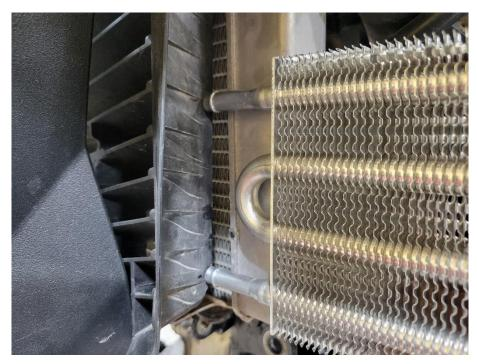
**Step 4.** Using a step bit or drimmel tool, trim out 2 holes in the radiator grill for the fluid cooler hoses to have clearance. You will need to trim more than you think to clear the 3/8" hoses.
