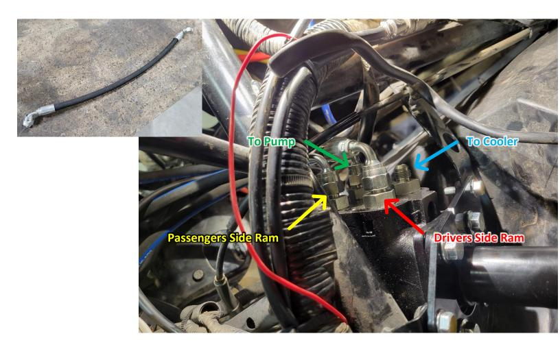
**Step 4.** Now, connect the lower low-pressure hose from the cooler to the return barb on the pump and secure with the supplied hose clamp. Also connect the high-pressure hose from the orbital to the pump and tighten.
