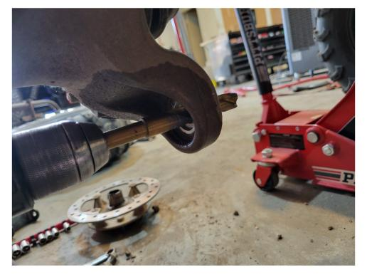
Once the rear hub assembly has been modified the new ball joint will install perfectly.
