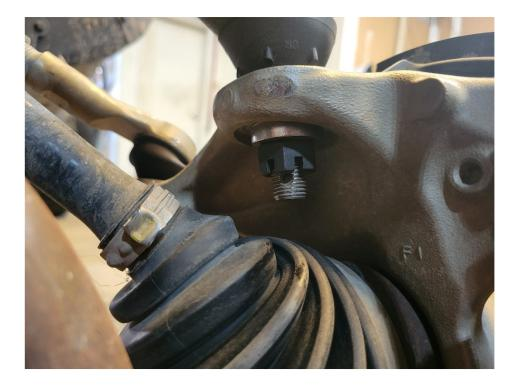
**Step 5. (Install Upper Control Arm Into the Hub Assembly)** Remove the cotter pin and castle nut from the Moog upper ball joint and install it into the hub assembly. Make sure to only tighten the castle nut hand tight until front installation is complete and desired camber is achieved. Do not install cotter pin at this time.
