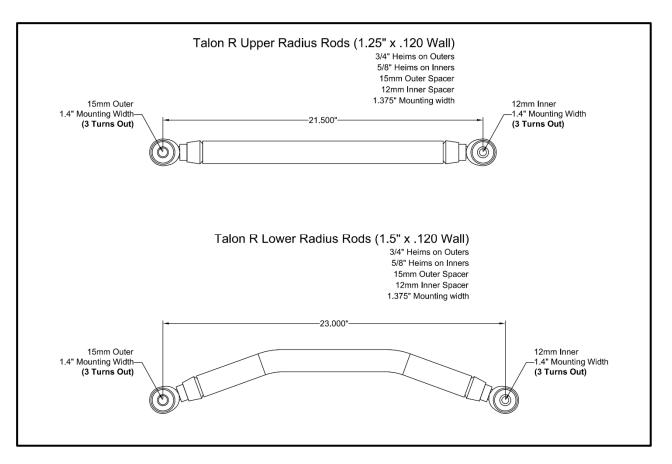
Once eye to eye dimensions are confirmed, install TTC Radius Rods onto the machine, using all factory mounting hardware.
