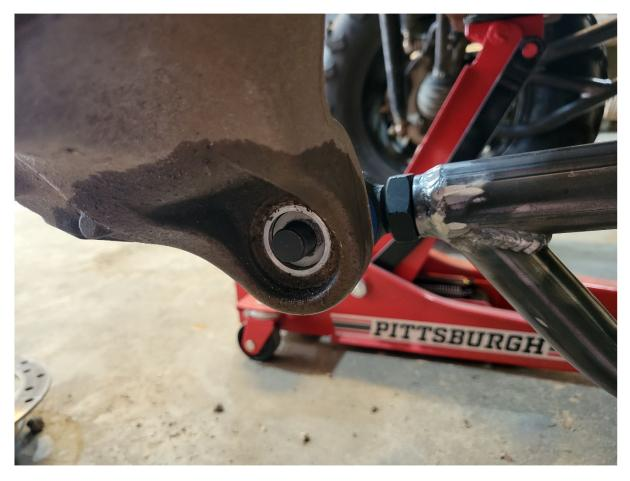
Using the stock hardware, reinstall your new TTC Arms back on the machine and repeat on other side.
