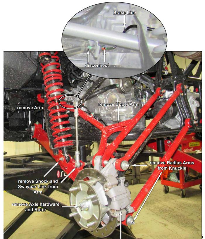
remove Caliper from Knuckle
