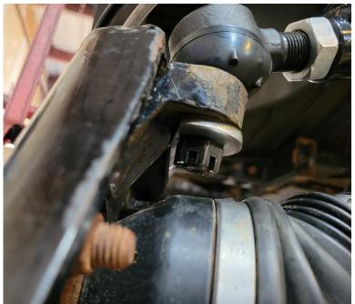
**Step 7. (Install Shock)** Before installing the front shock you must first install the supplied front coil spring spacer to insure that your stock shocks do not bottom out during operation (unless you are running aftermarket adjustable shocks). To do so compress your factory springs until you can remove the top factory retaining clip on the top of the spring.
