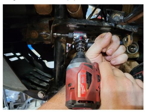
**Step 2. (Tack in New Tabs)** Using the new TTC 2 Bolt Design arm and provided 12mm nuts & bolts, install arm into existing space like the picture below. Install the new weld in frame tabs at this time and secure everything hand tight with the provided hardware. Once everything is fitted evenly and where you want it, tack it in. **(Make sure to remove the arm quickly so you don't melt the UMHW bushings)**
