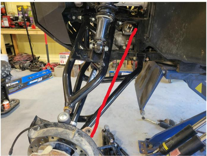
Next, make sure the jam nut is not installed on the inner tie rod (or heim joint), and push your stock tie rod boot on to the 14 mm shaft of the inner tie rod end. Make sure the boot is properly installed and seated in the groove on the rack and pinon, then secure it tightly with a zip tie.
