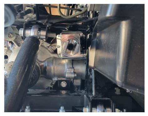
Next, make sure the jam nut is not installed on the inner tie rod (or heim joint), and push your stock tie rod boot on to the 14 mm shaft of the inner tie rod end, then screw on the jam nut. Make sure the boot is properly installed and seated in the groove on the rack and pinon, then secure it tightly with a zip tie.
