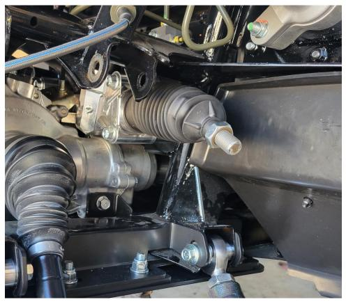
Next, screw on the jam nut, then screw the HD tie rod all the way on to the inner tie rod that was previously installed into the rack and pinion. Secure the tie rod assembly out of the way until a later step.
