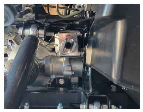
Next, make sure the jam nut is not installed on the inner tie rod (or heim joint), and push your stock tie rod boot on to the 14 mm shaft of the inner tie rod end. Make sure the boot is properly installed and seated in the groove on the rack and pinon, then secure it tightly with a zip tie.
