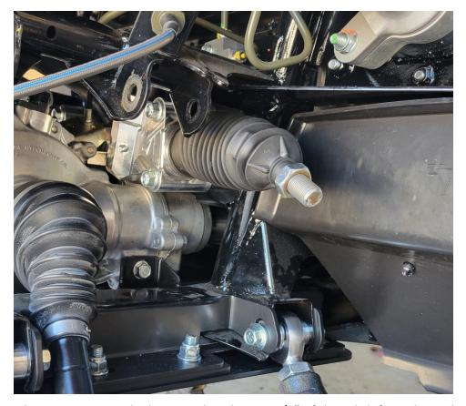
Next, screw the jam nut on to the heim so that there is 3/4" of threads left on the end of the heim, then screw the HD tie rod all the way up to the jam nut. Secure the tie rod assembly out of the way until a later step.
