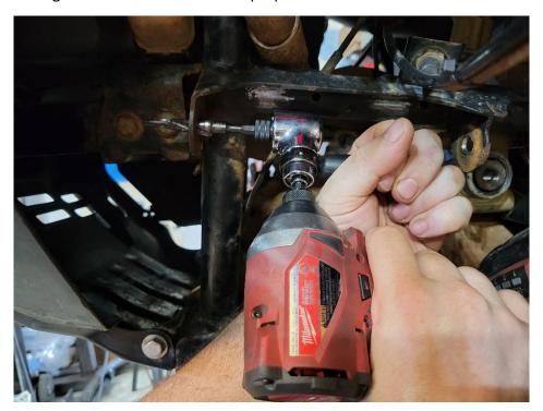
**Step 2. (Tack in New Tabs)** Using the new TTC 2 Bolt Design arm and provided 12mm nuts & bolts, install arm into existing space like the picture below. Install the new weld in frame tabs at this time and secure everything hand tight with the provided hardware. Once everything is fitted evenly and where you want it, tack it in. **(Make sure to remove the arm quickly so you don't melt the UMHW bushings)**
