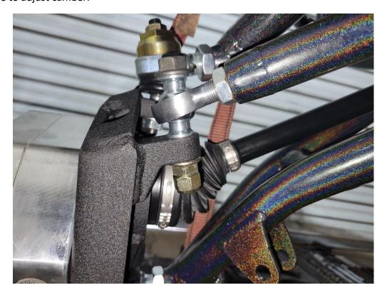
**Step 8. (Tighten Frame Bolts)** Once everything is assembled hand tight, go ahead and fully tighten both the upper and lower frame bolts that mount the control arms to the frame.
