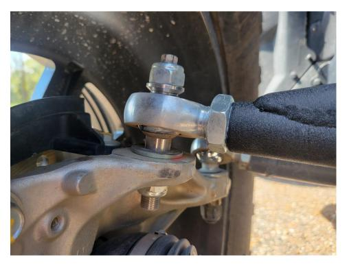
If you are running our heim style ball joint setup, first use a 10mm wrench to hold the pin, and tighten down the top locking nut on to the heim (**no need to over tighten**). Then insert the pin into the hub assembly and tighten the lower nut while holding the top of the pin with a 10mm wrench (**no need to over tighten**).
