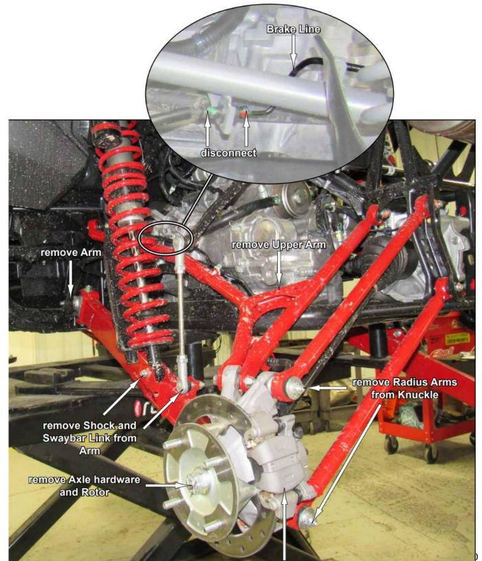
remove Caliper from Knuckle
