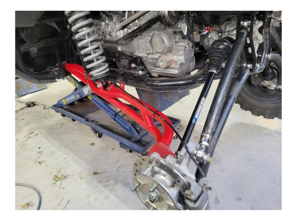
It is recommended to remove at least 1" of preload on the rear shocks from the factory settings. This will lower the rear of the machine and help soften the rear end buck that the Talon X is known for.
