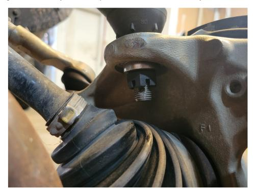
**Step 5. (Install Upper Control Arm Into the Hub Assembly)** Remove the cotter pin and castle nut from the Moog upper ball joint and install it into the hub assembly. Make sure to only tighten the castle nut hand tight until front installation is complete and desired camber is achieved. Do not install cotter pin at this time.
