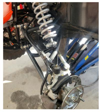
Once both sides are complete, re-install the tires and lower the machine to the ground. Start it up and pull it forward and back while turning the wheels back and forth to allow the shocks to settle to true ride height. Once the suspension has settled back down to normal, check to see if you have achieved the desired camber (wheels are straight up and down).
