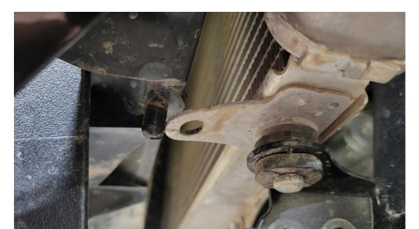
**Step 3.** Now locate the fluid cooler and use it to mark the radiator grill for trimming.
