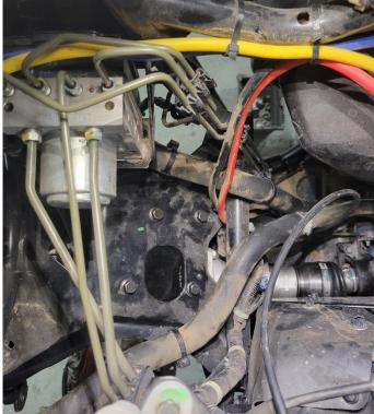
**Step 2.** Locate the 2 hydraulic lines that go from the ram to the orbital valve and install them. One end will have a 1/4" fitting for the ram side, and the other will have a 3/8" fitting for the orbital side.
