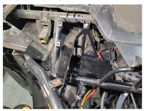
`**Step 3.** Next, locate the pump to orbital valve hose shown below. First connect one end to the orbital valve and tighten down. Route the other end up to pump area. At this time go ahead and connect the hose barb from the Upper Fluid cooler hose to the last spot on the orbital valve and tighten down.
