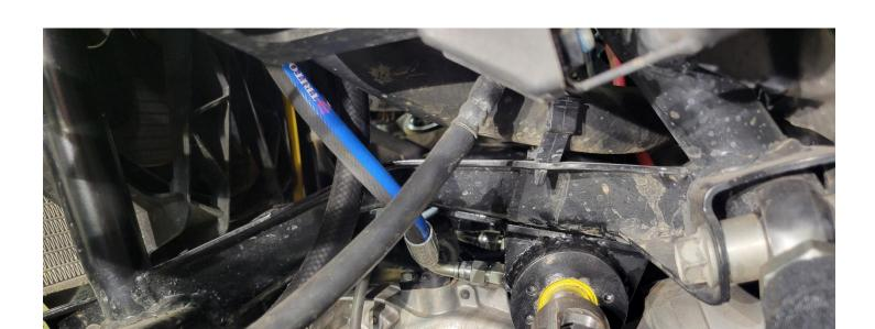
Ideally you want to line the clevis "ears" up with the hole in the hub assembly where the outer tie rod will attach. See pic below.
