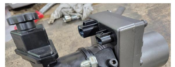
**Step 2.** Now install the TTC pump bracket/battery tray as shown below.
