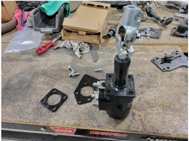
Make sure the notch in the mounting bracket is in the same direction as the orbital valve ports.
