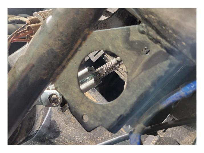
**Step 5.** Once you get the shaft in place, install the bottom 2 frame bolts. The top bolt will need to be trimmed down so that it is 1/2" long. (See pic below)
