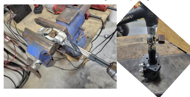
**Step 3.** Now assemble the Orbital valve in this order, steering column, bracket spacer, frame bracket. For now, leave the bolts hand tight. Install and tighten the fittings into the Orbital valve at this time.
