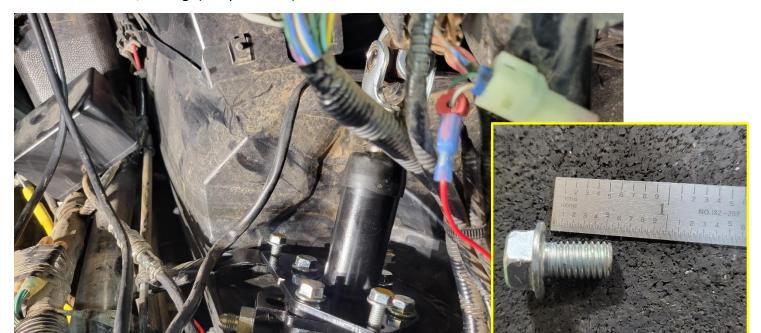
**Step 6.** Once everything is in place, tighten down the 3 bolts that secure the orbital valve bracket to the frame. Then tighten down the 4 bolts that hold the bracket and steering column to the orbital valve. **(Don't worry about whether your steering wheel is straight or not at this time)**
