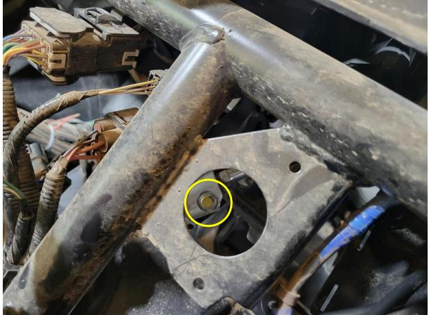
**Step 3.** Once you have removed the steering shaft bolts, disconnect the 2 electrical connectors from the EPS unit. Next remove the 3 bolts that mount the EPS unit to the frame, and remove the EPS unit from the machine along with the steering yolk.
